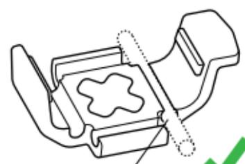
Strap fitted securely in mount groove
